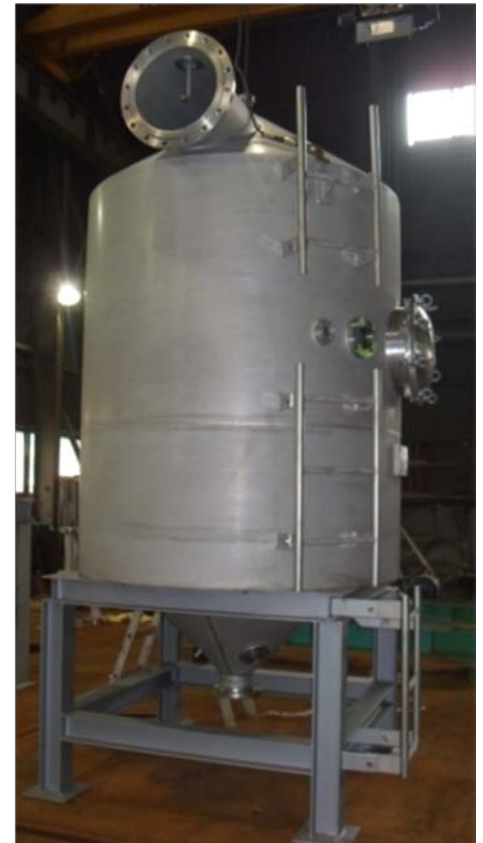
Flash vessel on frame delivered by EPCON as part of project with engineering and component delivery.
