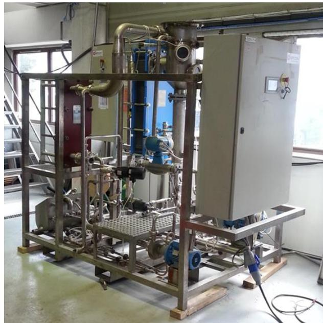
All the mobile evaporation test rigs are highly automated. Fluid feed, concentration, temperature and pressure are controlled automatically, and values displayed on the operator's monitor. The test units can be connected to internet to enable remote monitoring and control from EPCON's offices.
