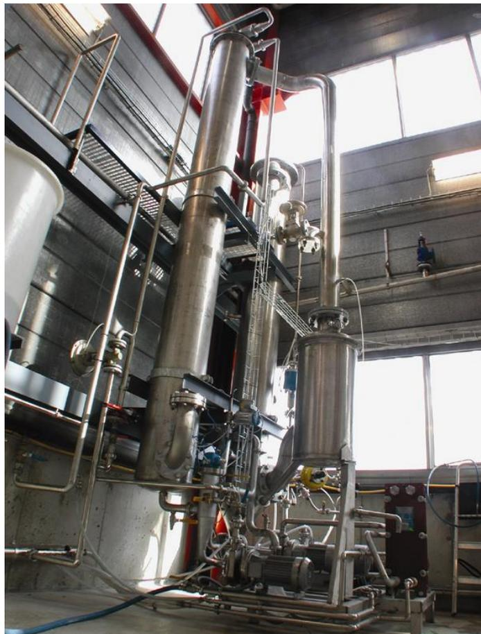
The test rig is highly automated. Fluid feed, concentration, temperature and pressure are controlled automatically, and values displayed on the operator's monitor.
