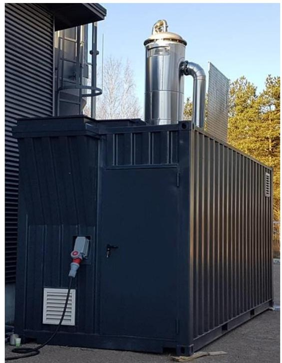
All the mobile test rigs are highly automated. Fluid feed, concentration, temperature and pressure are controlled automatically, and values displayed on the operator's monitor. The test units can be connected to an analogue telephone line to enable remote monitoring and control from EPCON's offices.
