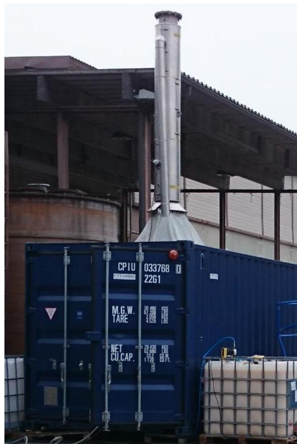
All the mobile test rigs are highly automated. Fluid feed, concentration, temperature and pressure are controlled automatically, and values displayed on the operator's monitor. The test units can be connected to an analogue telephone line to enable remote monitoring and control from EPCON's offices.
